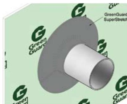
FIGURE 10C: INSTALLATION OF FLASHING PIPE PENETRATION
