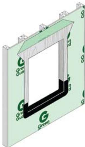
FIGURE 4B: INSTALLATION OF SILL FLASHING AND CUT BACK OF WRAP ON THE SIDES
