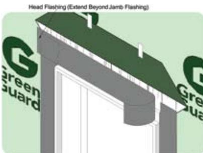
FIGURE 3C: INSTALLATION OF WINDOW HEAD FLASHING
